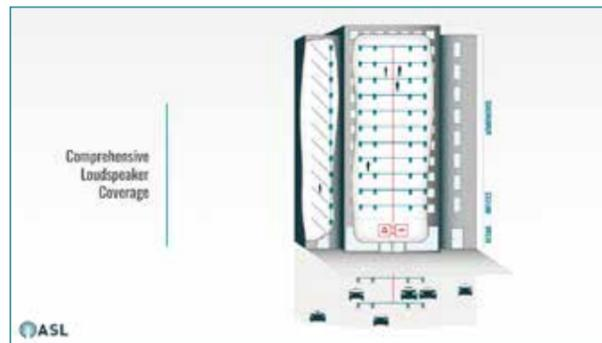
Loudspeakers are installed on each floor with separate zones for the staircases, all connected to a single Fire Panel and VACIE on the ground floor.
