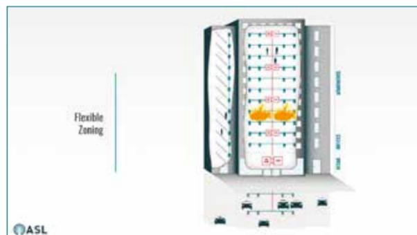
By deploying a distributed system with redundancy i.e. double cabling, multiple fire panels and VACIE systems, the system becomes much more flexible and resilient to stress / building damage.
