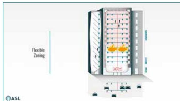
In this example of a traditional system it appears to work well, unless the system becomes compromised by the fire and the higher floors become isolated from the VACIE system messaging.
